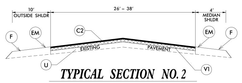
\*Note Mill and Fill between rumble strips and fog seal paved shoulder
