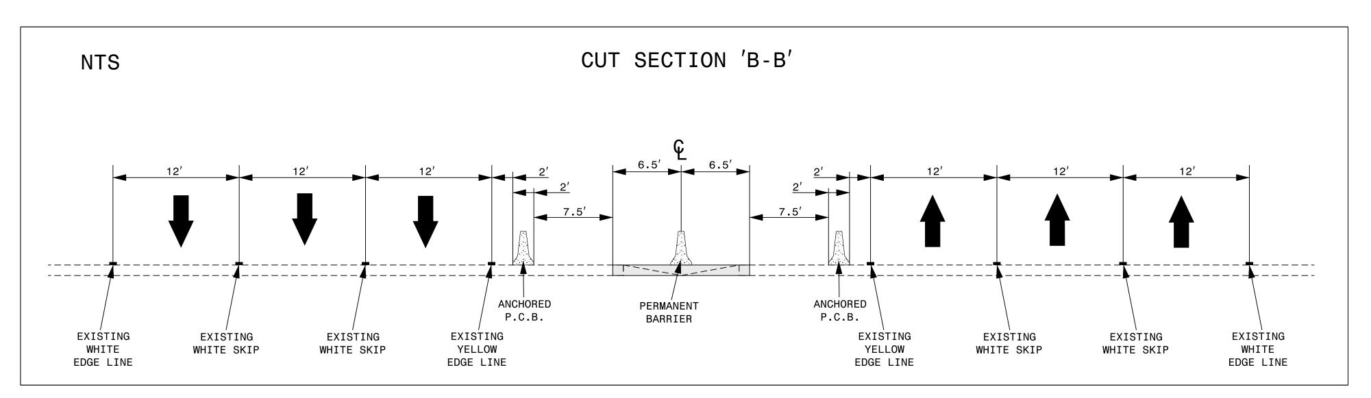
REFER TO RSD 1101.05, SHEET 2 FOR WORK ZONE VEHICLE INGRESS/EGRESS THROUGH P.C.B. COORDINATE WITH AND OBTAIN ENGINEER'S APPROVAL OF ACCESS POINTS TO/FROM MEDIAN WORK AREA. THERE SHALL BE NO MORE THAN ONE WORK ZONE VEHICLE ACCESS THROUGH P.C.B. PER TRAVEL DIRECTION WEST OF LEWISVILLE CLEMMONS ROAD AND NO MORE THAN ONE WORK ZONE VEHICLE ACCESS THROUGH P.C.B. PER TRAVEL DIRECTION EAST OF LEWISVILLE CLEMMONS ROAD.
