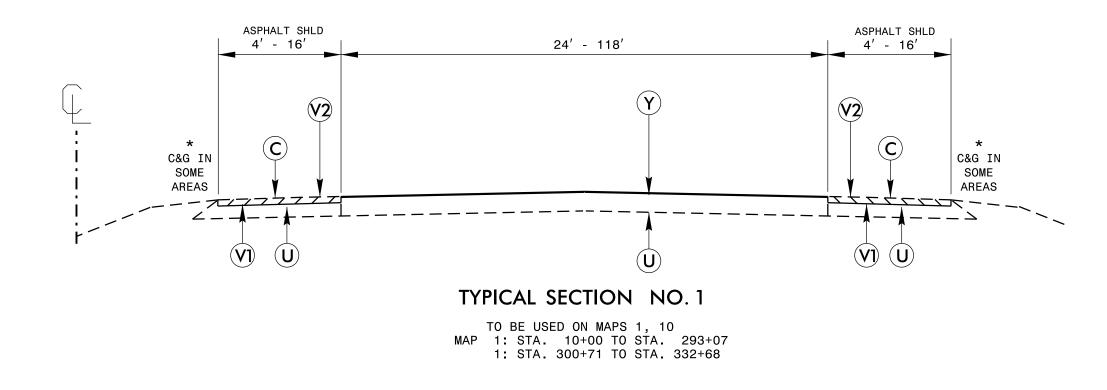
CONTRACTOR SHALL PERFORM MILL/FILL OPERATION ON SHOULDER BEFORE DIAMOND GRINDING TO AVOID TACK AND DEBRIS ON FINAL CONCRETE PAVEMENT SURFACE. DIAMOND GRIND EXISTING TRAVEL LANES, AUXILIARY LANES AND RAMPS INCLUDING GORE AREAS DIAMOND GRINDING OPERATION SHALL BE PERFORMED AFTER ALL CONCRETE REPAIRS ARE COMPLETE AND PRIOR TO JOINT SEALING OPERATION
