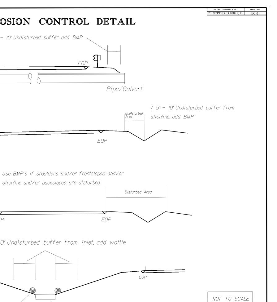
NOTES: Less than 5' - 10' undisturbed buffer from ROW, ditchline, water feature, or drainage inlet, add BMP.
