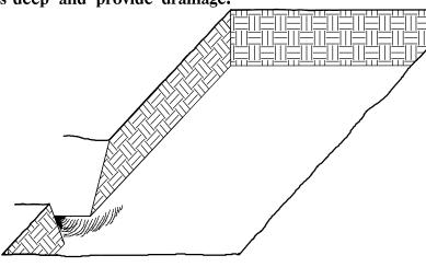
3. Jackfill the trench with 2 inches well rotted sawdust. Place a 2 inch layer of well rotted sawdust at a sloping angle at one end of the trench.
