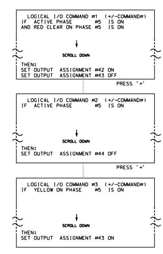
LOGIC I/O PROCESSOR PROGRAMMING COMPLETE
