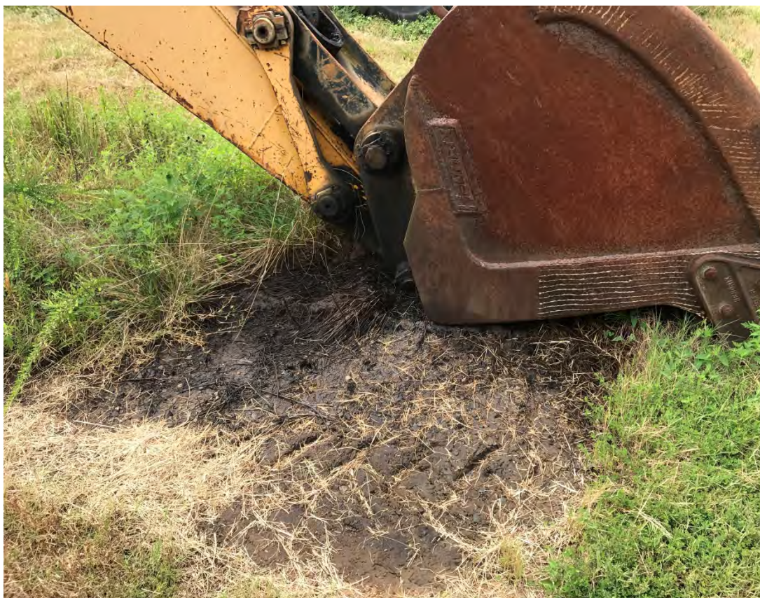
Photograph No. 6 View of impacted soil from leaking hydraulic line on excavation equipment.
