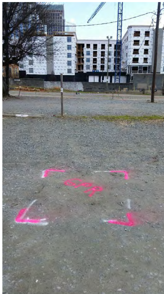
Photo 17: Showing GPR anomaly in Parcel 5B.
