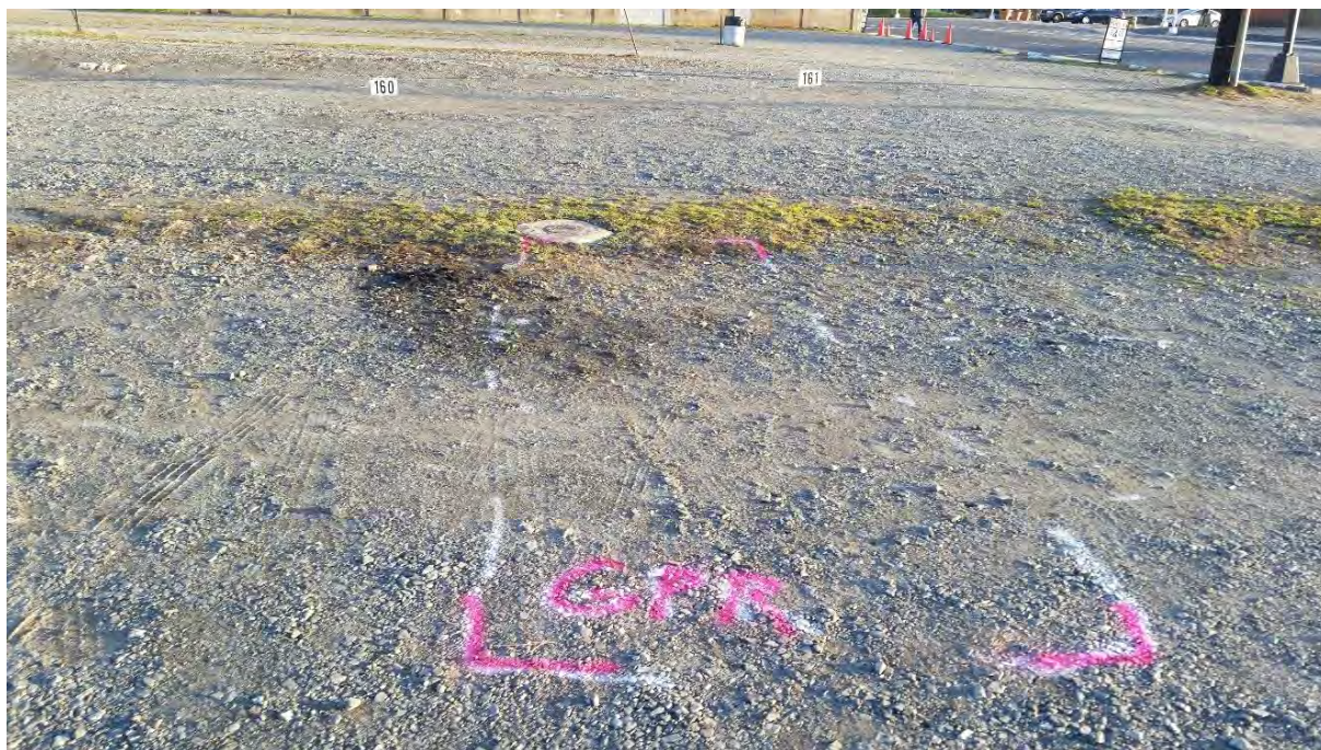
Photo 10: Showing GPR anomaly and monitoring well in Parcel 6.
