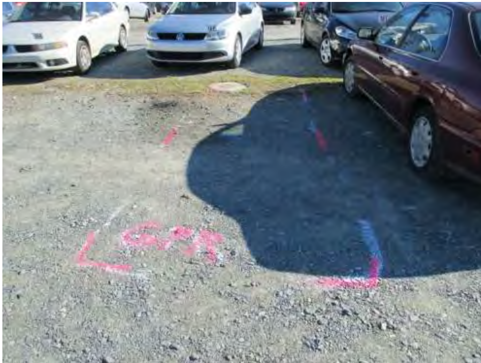
Photo 7 View of the GPR/EM markings with monitoring well in the grass.
