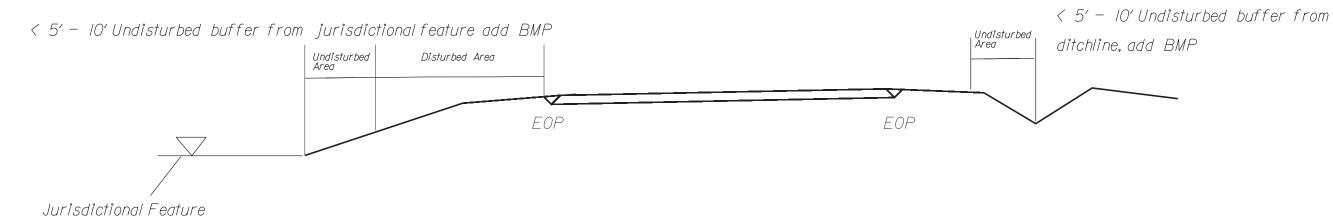
Use BMP's if shoulders and/or frontslopes and/or ditchline and/or backslopes are disturbed
