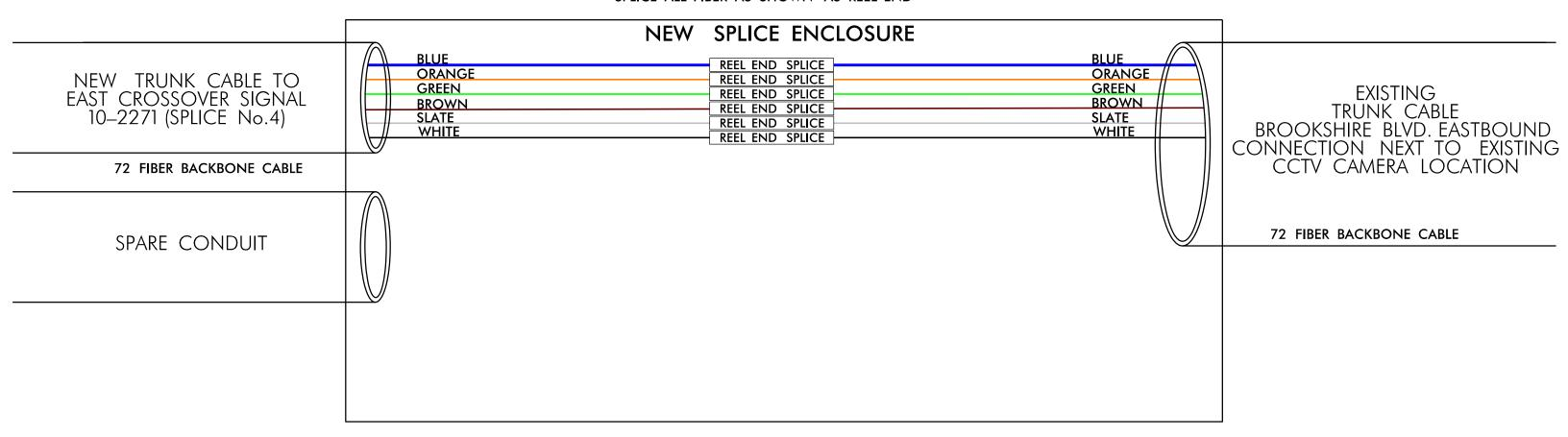
INCLUDE ON THE COVER OF EACH SPLICE TRAY THE FOLLOWING: REFERENCE SECTION 1731 "FIBER OPTIC SPLICE ENCLOSURE" 1) SPLICE LOCATION 2) DATE 3) COMPANY NAME 4) NAME OF INDIVIDUAL PERFORMING THE SPLICING PRIOR TO INSTALLING THE COVER ON THE SPLICE TRAY TAKE A DIGITAL PHOTOGRAPH SHOWING THE SPLICE TRAY AND INFORMATION SHOWN ABOVE (1-4) AND SUBMIT PHOTOGRAPH ALONG WITH OTDR TEST RESULTS.
