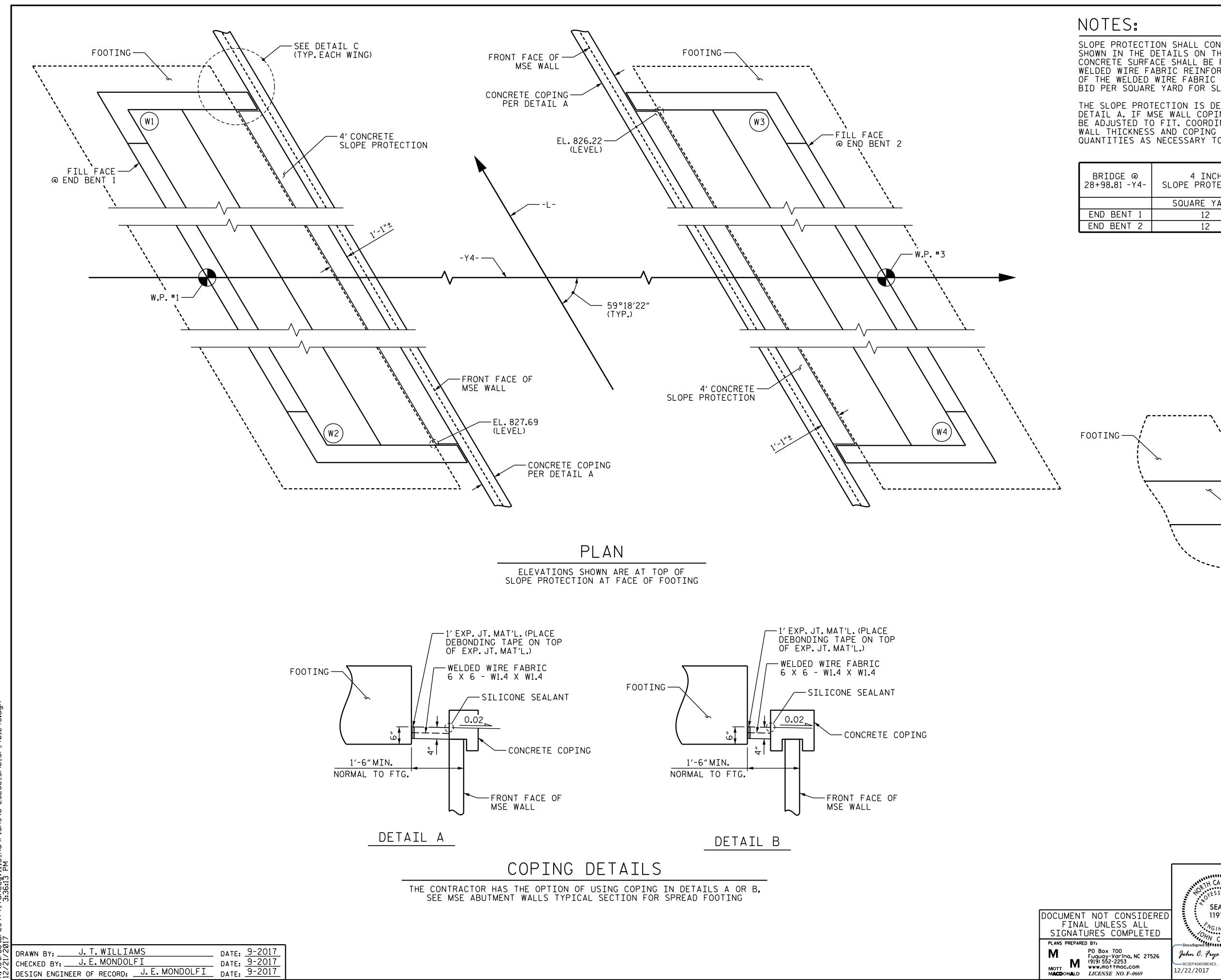
SLOPE PROTECTION SHALL CONSIST OF 4" POURED-IN-PLACE CONCRETE PAVING AS SHOWN IN THE DETAILS ON THIS SHEET. CONCRETE SHALL BE CLASS "B". THE CONCRETE SURFACE SHALL BE FLOATED WITH A WOODEN FLOAT AND FINISHED. WELDED WIRE FABRIC REINFORCING SHALL BE 6 X 6 - W1.4 X W1.4. THE COST OF THE WELDED WIRE FABRIC SHALL BE INCLUDED IN THE CONTRACT UNIT PRICE BID PER SQUARE YARD FOR SLOPE PROTECTION.
