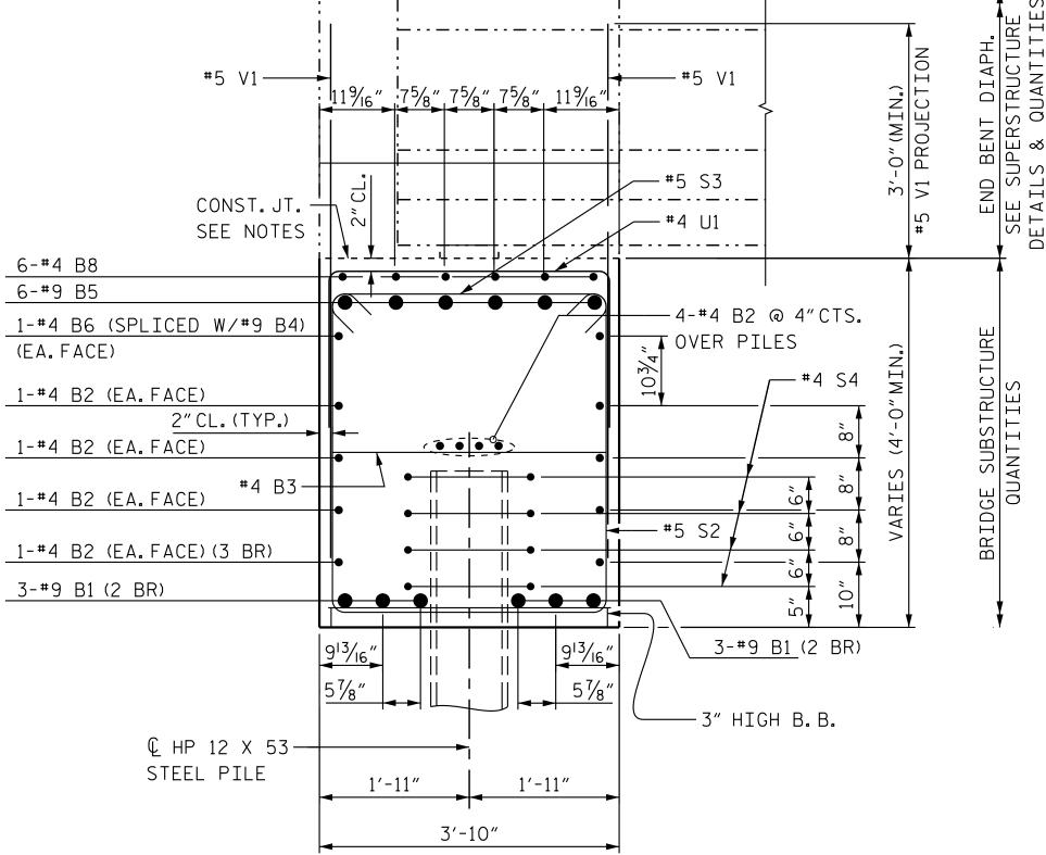
SECTION A-A SEE "END BENT 1" SHEET 1 OF 3 scaled up by 1.5
