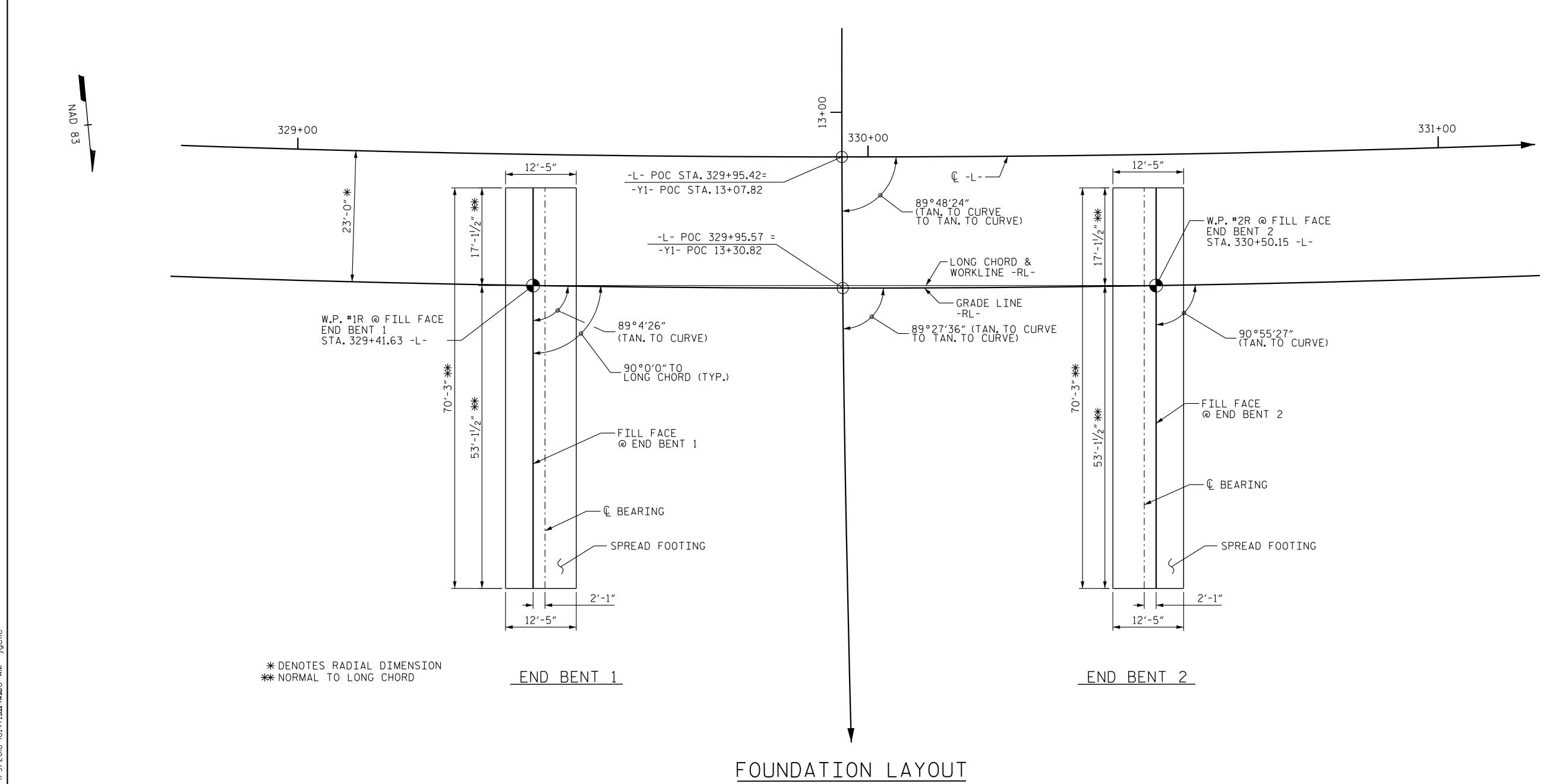
NOTE: ALL SUBSTRUCTURE WORK LINES PASS THROUGH WORK POINTS.
