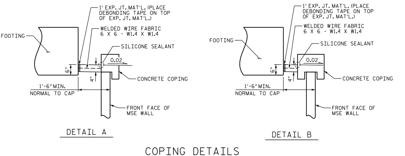
THE CONTRACTOR HAS THE OPTION OF USING COPING IN DETAILS A OR B,
