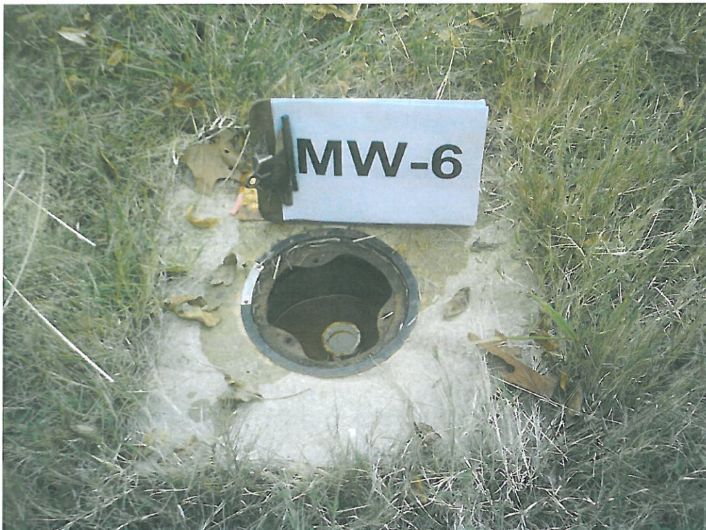
Photograph 4: Typical monitoring well prior to abandonment
