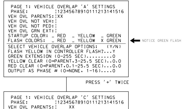
VEH OVL NOT VEH: | VEH OVL NOT PED: VEH OVL GRN EXT: STARTUP COLOR: \_ RED \_ YELLOW \_ GREEN FLASH COLORS: \_ RED \_ YELLOW X GREEN NOTICE GREEN FLASH SELECT VEHICLE OVERLAP OPTIONS: (Y/N) FLASH YELLOW IN CONTROLLER FLASH?...Y GREEN EXTENSION (0-255 SEC).....0 YELLOW CLEAR (O=PARENT,3-25.5 SEC)..0.0 RED CLEAR (0=PARENT,0.1-25.5 SEC)...0.0 OUTPUT AS PHASE # (0=NONE, 1-16)....0
