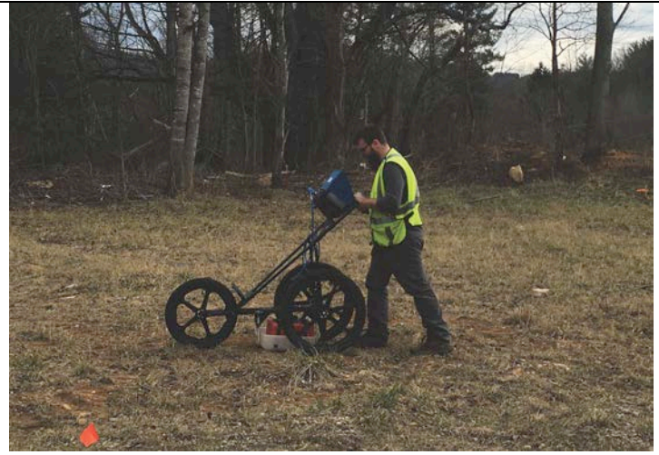
GPR data collection in Grid 1 across the footprint of the former building.
