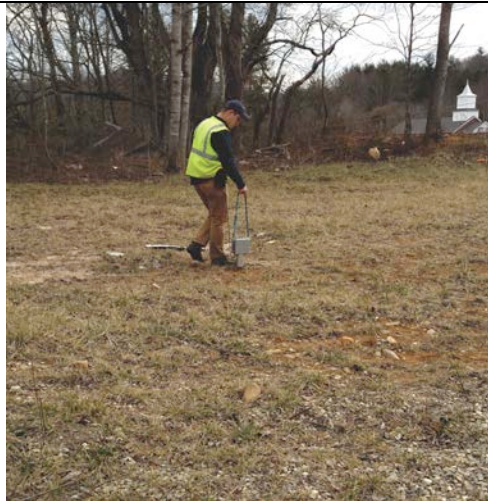
Magnetometer data collection in Grid 1 across the footprint of the former building.
