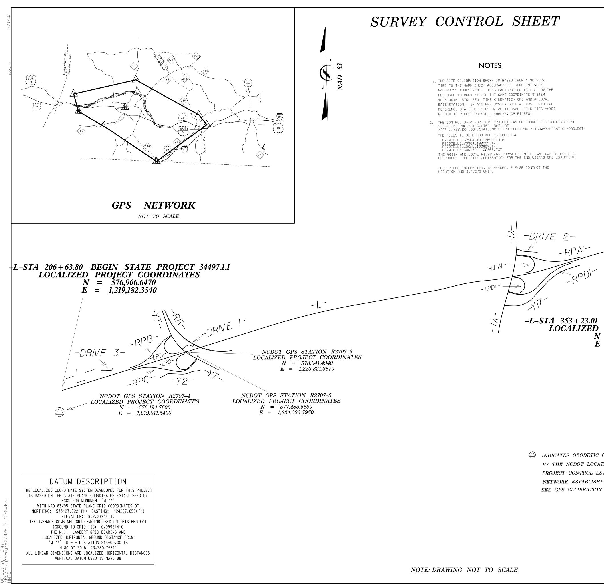
INDICATES GEODETIC CONTROL MONUMENTS USED OR SET FOR HORIZONTAL PROJECT CONTROL BY THE NCDOT LOCATION AND SURVEYS UNIT. PROJECT CONTROL ESTABLISHED UTILIZING GLOBAL POSITIONING SYSTEM. NETWORK ESTABLISHED FROM EXISTING HARN MONUMENTATION. SEE GPS CALIBRATION SHEET FOR HORIZONTAL AND VERTICAL COORDINATE VALUES
