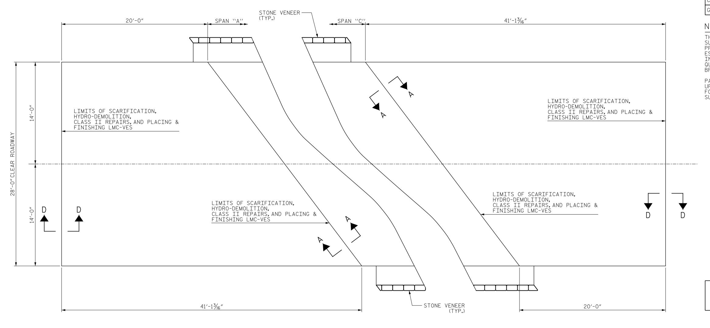
SUMMARY OF QUANTITIES FOR WEST APPROACH ESTIMATE ACTUAL SCARIFYING BRIDGE DECK 95.0 SY HYDRO-DEMOLITION OF BRIDGE DECK 95.0 SY CLASS II SURFACE PREPARATION GROOVING BRIDGE DECK 786.7 SUMMARY OF QUANTITIES FOR EAST APPROACH ESTIMATE ACTUAL SCARIFYING BRIDGE DECK 95.0 SY HYDRO-DEMOLITION OF BRIDGE DECK 95.0 SY CLASS II SURFACE PREPARATION 786.7 GROOVING BRIDGE DECK
