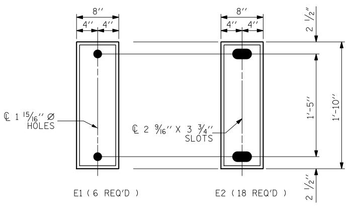
PLAN VIEW OF ELASTOMERIC BEARING
