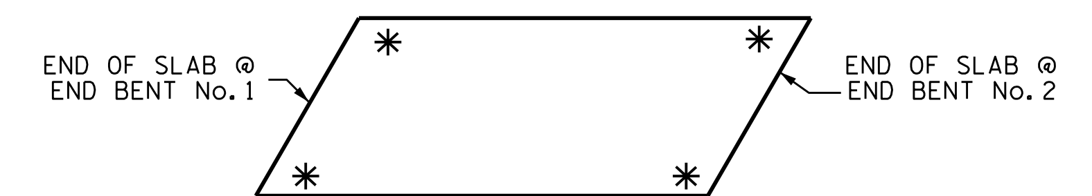
SKETCH SHOWING POINTS OF ATTACHMENT
