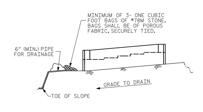
BAGGED STONE AND PIPE SHALL BE PLACED IMMEDIATELY AFTER COMPLETION OF END BENT EXCAVATION. PIPE MAY BE EITHER CONCRETE, CORRUGATED STEEL, CORRUGATED ALUMINUM ALLOY, OR CORRUGATED PLASTIC. PERFORATED PIPE WILL NOT BE ALLOWED.
