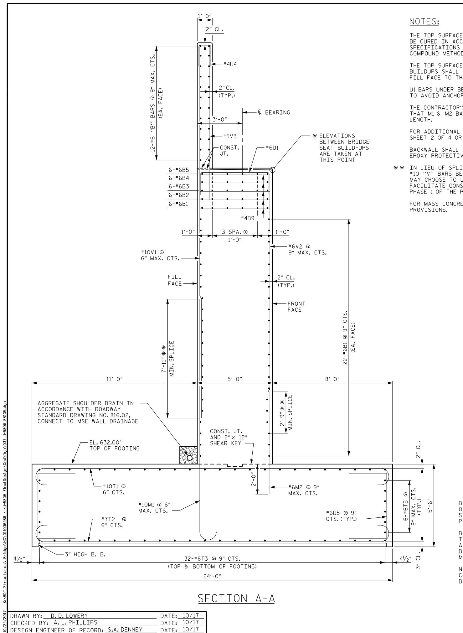
THE TOP SURFACE AREAS OF THE END BENT CAP SHALL BE CURED IN ACCORDANCE WITH THE STANDARD SPECIFICATIONS EXCEPT THAT THE MEMBRANE CURING COMPOUND METHOD SHALL NOT BE USED.
