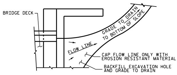
IF THE APPROACH SLAB IS NOT CONSTRUCTED IMMEDIATELY AFTER THE BACKFILLING OF THE END BENT EXCAVATION, GRADE TO DRAIN TO THE BOTTOM OF THE SLOPE AND PROVIDE EROSION RESISTANT MATERIAL, SUCH AS FIBERGLASS ROVING OR AS DIRECTED BY THE ENGINEER TO PREVENT SOIL EROSION AND TO PROTECT THE AREA ADJACENT TO THE STRUCTURE.
