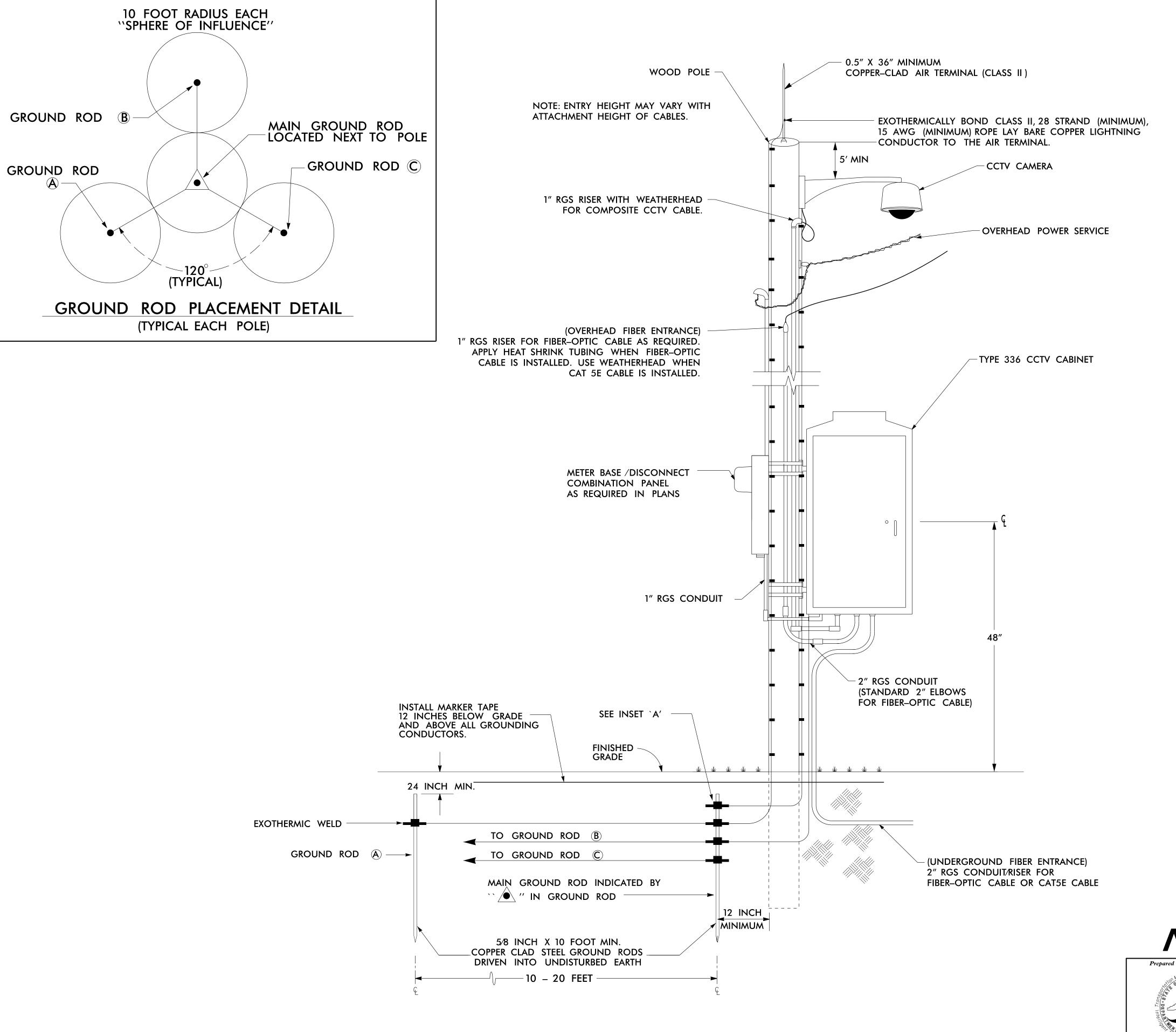
INSET `A' SCP-04 U-4751 #4 AWG SOLID BARE COPPER WIRE TO GROUND RODS A, B, AND C CLASS II COPPER CONDUCTOR TO AIR TERMINAL **#4 AWG SOLID BARE COPPER** WIRE TO CAMERA SUPPORT BASE #4 AWG SOLID BARE COPPER -WIRE TO EXTERNAL DISCONNECT GROUND BUS
