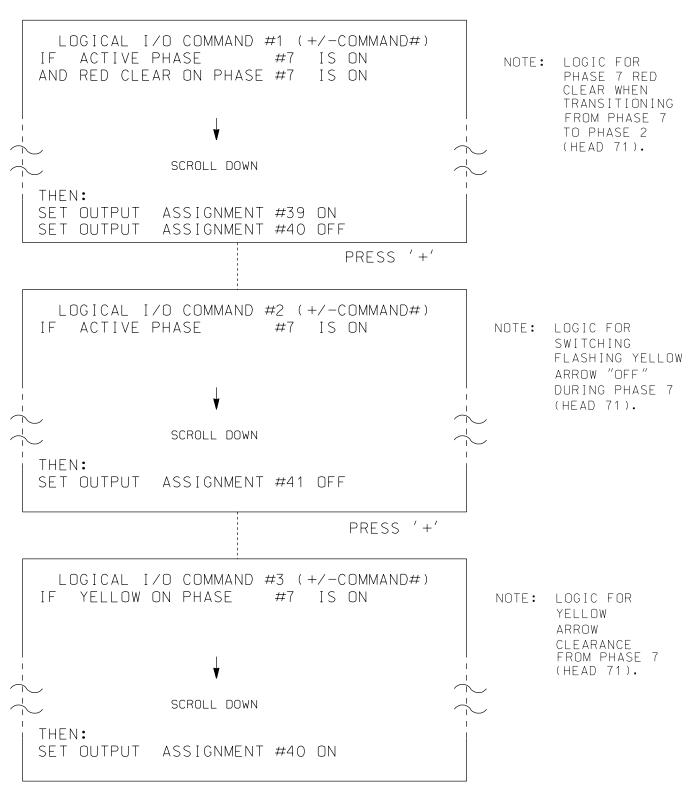
LOGIC I/O PROCESSOR PROGRAMMING COMPLETE
