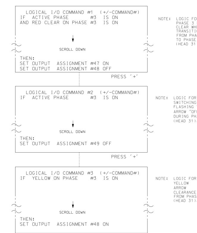
LOGIC I/O PROCESSOR PROGRAMMING COMPLETE
