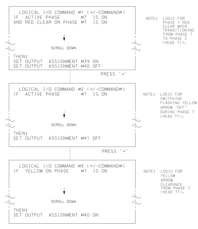
LOGIC I/O PROCESSOR PROGRAMMING COMPLETE
