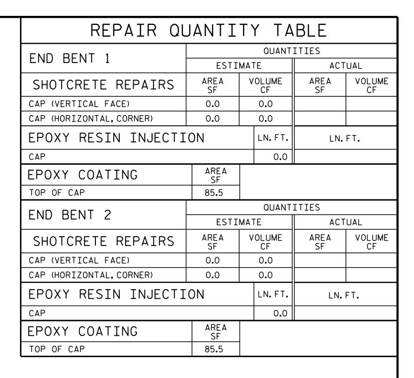
REPAIR LOCATIONS AND ESTIMATE OF QUANTITIES ARE GIVEN WITH THE BEST INFORMATION AVAILABLE. IF ADDITIONAL REPAIRS NOT SHOWN ON THE DRAWINGS ARE DEEMED NECESSARY BY THE INSPECTOR OR ENGINEER THE CONTRACTOR SHALL NOTE ON THE DRAWINGS THE APPROXIMATE LOCATION AND DESCRIPTION OF THE REPAIRS AND ADJUST THE ACTUAL QUANTITIES ENTERED INTO THE REPAIR QUANTITY TABLE.
