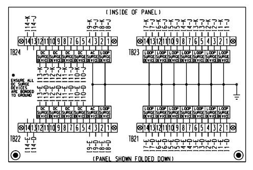
For base mounted cabinets, mount surge protection panels on the left side of the cabinet as viewed from the rear. Attach each panel to the cabinet rack assembly using bolts and make it easily removable. Mount the surge protection devices in vertical rows on each panel and connect the
