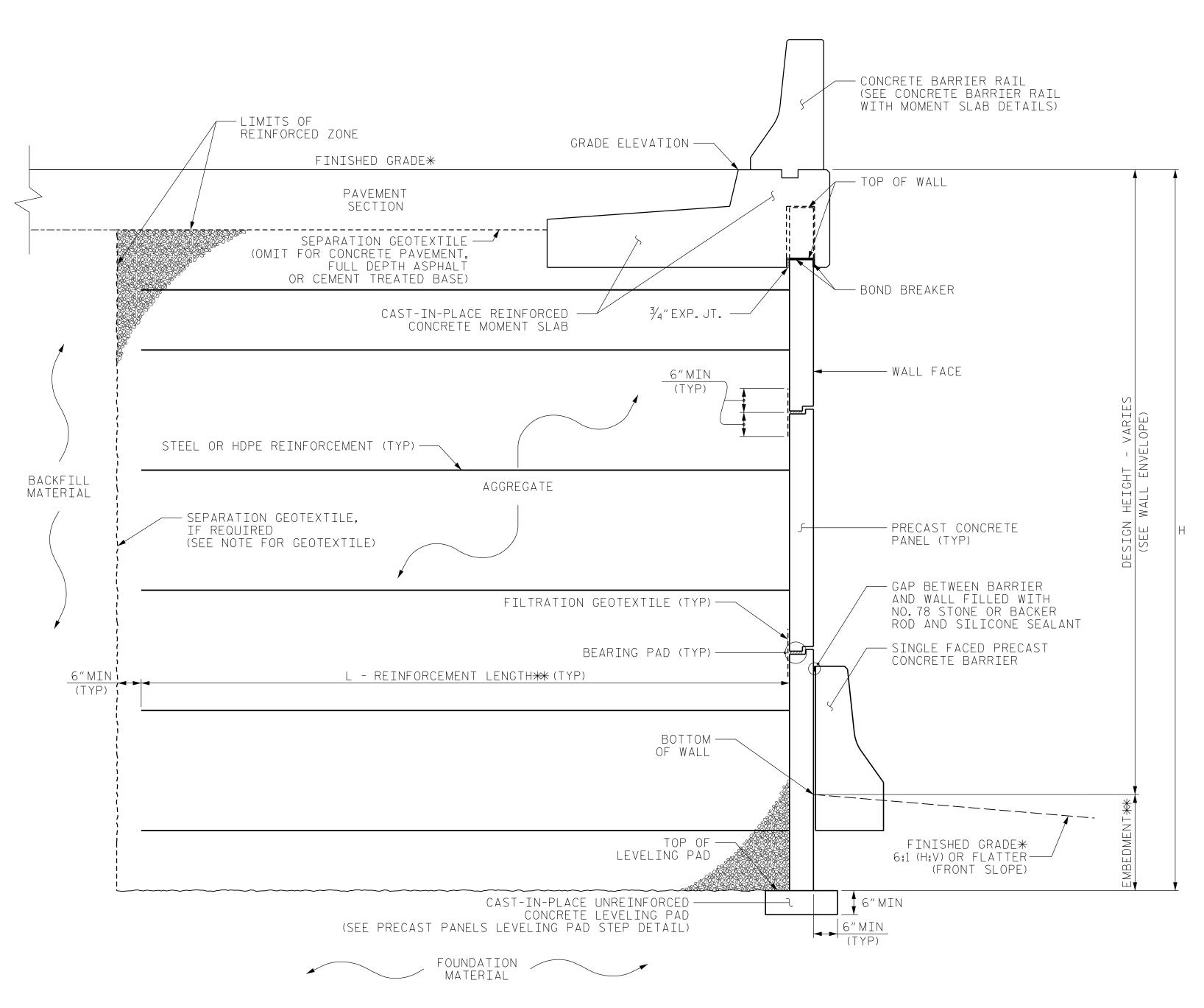
MSE WALL WITH PRECAST PANELS - TYPICAL SECTION
