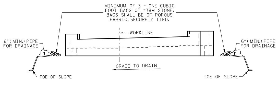
BAGGED STONE AND PIPE SHALL BE PLACED IMMEDIATELY AFTER COMPLETION OF END BENT EXCAVATION. PIPE MAY BE EITHER CONCRETE, CORRUGATED STEEL, CORRUGATED ALUMINUM ALLOY, OR CORRUGATED PLASTIC. PERFORATED PIPE WILL NOT BE ALLOWED.
