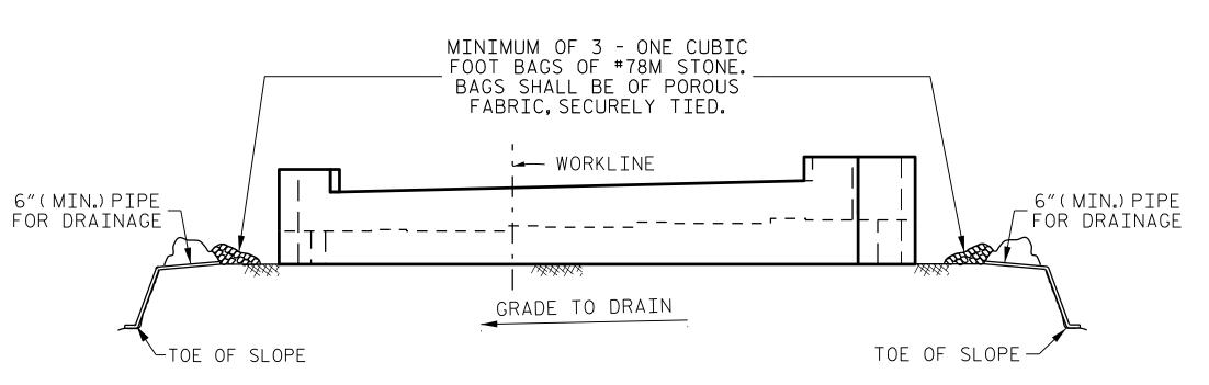
BAGGED STONE AND PIPE SHALL BE PLACED IMMEDIATELY AFTER COMPLETION OF END BENT EXCAVATION. PIPE MAY BE EITHER CONCRETE, CORRUGATED STEEL, CORRUGATED ALUMINUM ALLOY, OR CORRUGATED PLASTIC. PERFORATED PIPE WILL NOT BE ALLOWED.
