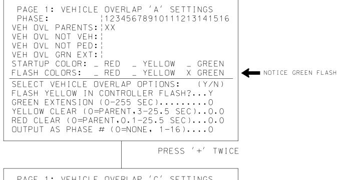
PAGE 1: VEHICLE OVERLAP 'C' SETTINGS 12345678910111213141516 PHASE: VEH OVL PARENTS: | XX VEH OVL NOT VEH: | VEH OVL NOT PED: 1 VEH OVL GRN EXT: | STARTUP COLOR: \_ RED \_ YELLOW \_ GREEN FLASH COLORS: \_ RED \_ YELLOW X GREEN SELECT VEHICLE OVERLAP OPTIONS: (Y/N) FLASH YELLOW IN CONTROLLER FLASH?...Y GREEN EXTENSION (0-255 SEC)..... YELLOW CLEAR (O=PARENT, 3-25.5 SEC)...O.O RED CLEAR (0=PARENT, 0.1-25.5 SEC)...0.0 OUTPUT AS PHASE # (0=NONE, 1-16)....
