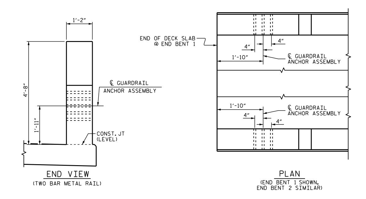
LOCATION OF GUARDRAIL ANCHOR AT END POST
