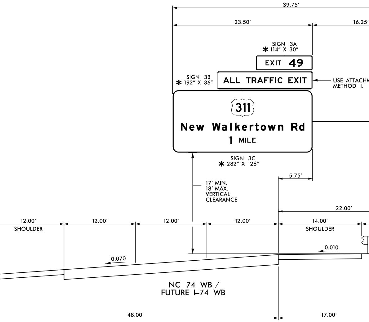
\* THESE DIMENSIONS SHALL BE USED FO WIND LOAD AND DEAD LOAD COMPU IN DESIGN OF STRUCTURE AND FOOTIN DESIGN AND CONSTRUCTION REQUIREM FOR SIGN STRUCTURES SHALL ACCOMODE WIND VELOCITY OF 90 M.P.H.
