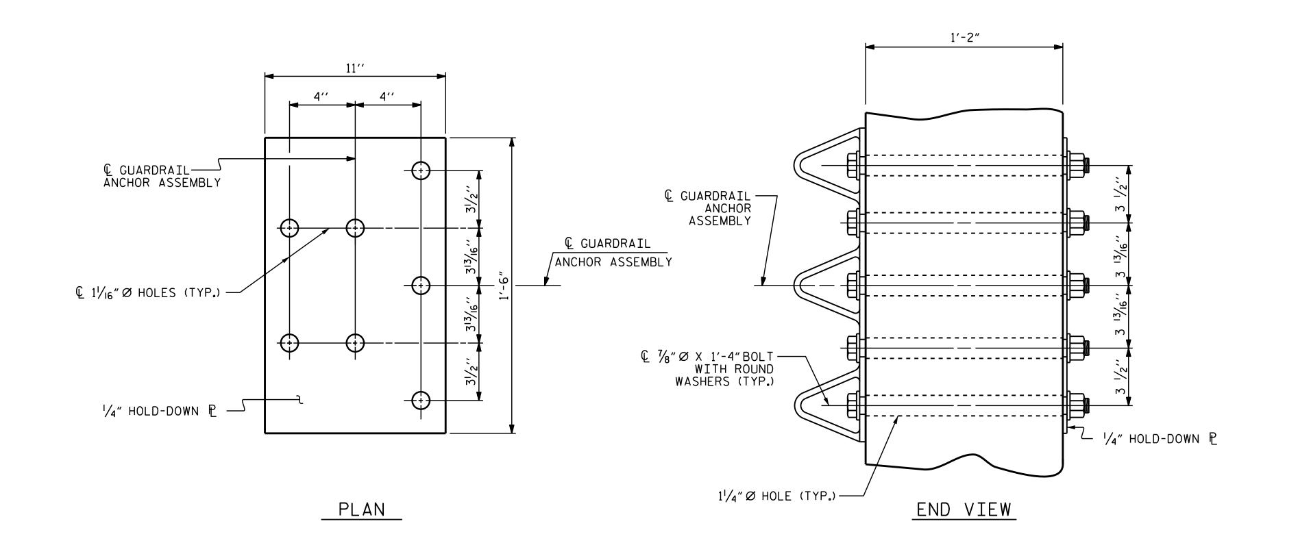
GUARDRAIL ANCHOR ASSEMBLY DETAILS
