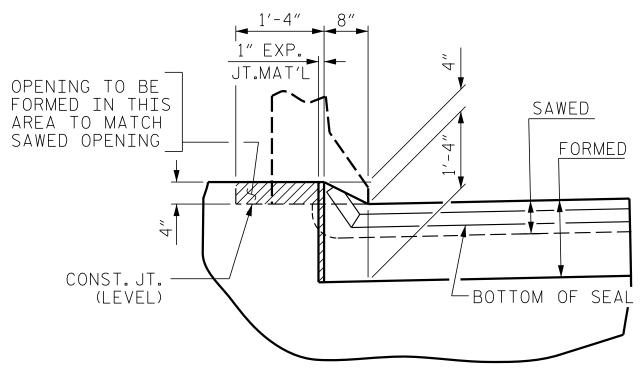
JOINT SEAL DETAILS @ END BENT
