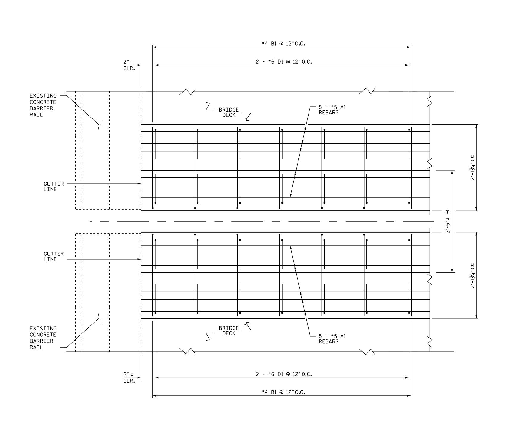
TYPICAL PLAN OF PROPOSED TOP REINFORCING (DECK SIDES)
