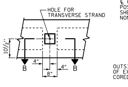
© 0.6" Ø L.R. TRANSVERSE POST-TENSIONING STRAND SHEATHED WITH A NON-CORROSIVE PIPE. OUTSIDE FACE -OF EXTERIOR CORED SLAB -WITH GROUT
