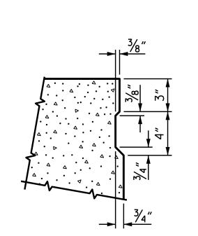
SHEAR KEY DETAIL NOTE: OMIT SHEAR KEY ON OUTSIDE FACE OF EXTERIOR CORED SLABS. PROJECT NO. B-5332 COLUMBUS COUNTY 12+67.50 -L-
