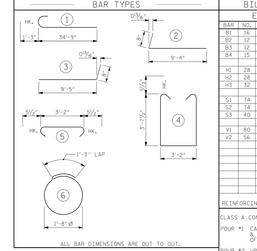
S1 | 74 | #5 11'-4" 875 S2 74 #5 4'-1" 315 S3 40 #4 6 6′-6″ 174 307 V1 | 80 | #4 | STR | 5′-9″ #4 | STR | 352 V2 | 56 9'-5" 5,243 LBS. REINFORCING STEEL CLASS A CONCRETE BREAKDOWN POUR #1 CAP, CONC. COLLARS 37.4 C.Y. & LOWER PART OF WINGS 5.2 C.Y. POUR #2 UPPER PART OF WINGS 42.6 C.Y. TOTAL CLASS A CONCRETE HP 12 X 53 STEEL PILES LIN.FT.= 850 NO: 10
