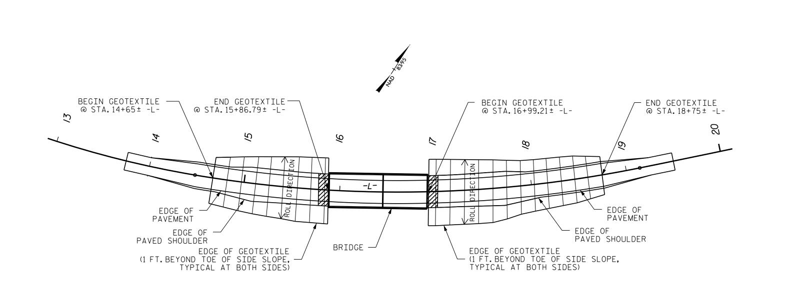
PLAN FOR GEOTEXTILE FOR EMBANKMENT STABILIZATION
