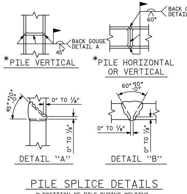
\* POSITION OF PILE DURING WELDING.
