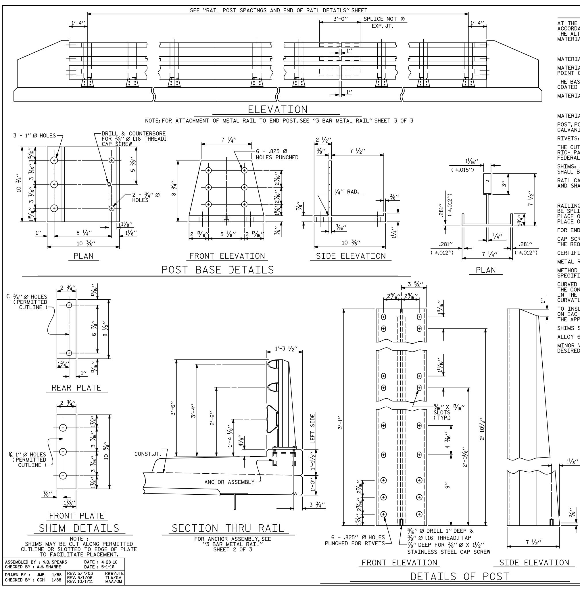
AT THE CONTRACTOR'S OPTION, METAL RAIL MAY BE EITHER ALUMINUM OR GALVANIZED STEEL IN ACCORDANCE WITH THE REQUIREMENTS OF THE GENERAL NOTES AND THE FOLLOWING SPECIFICATIONS FOR THE ALTERNATE MATERIALS; HOWEVER, THE CONTRACTOR WILL BE REQUIRED TO USE THE SAME RAIL MATERIAL ON ALL STRUCTURES ON THE PROJECT FOR WHICH METAL RAIL IS DESIGNATED.
