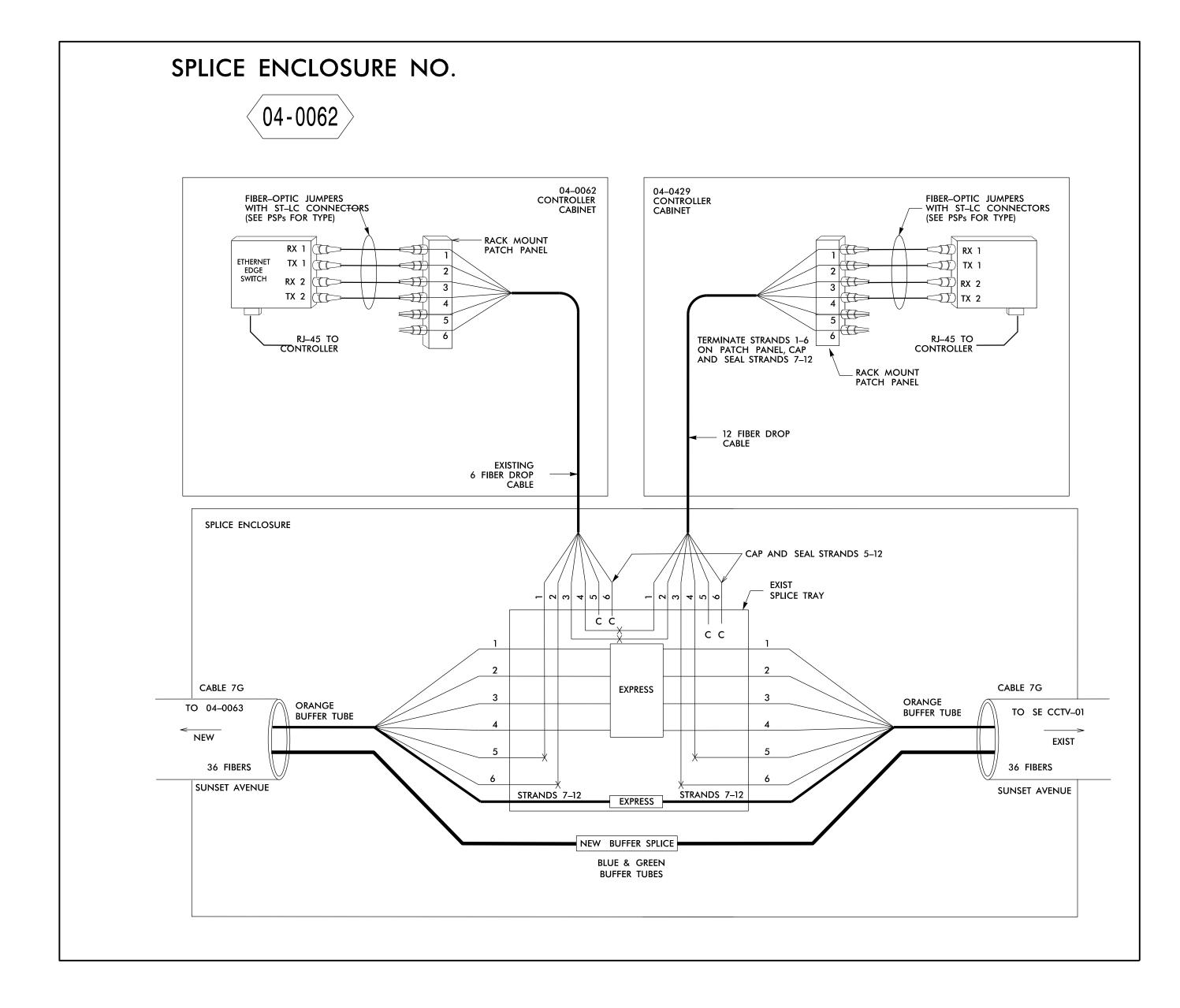
NOTE: MATCH CABLE NUMBER TO CORRESPONDING CABLE DESTINATION TO DETERMINE CORRECT DIAGRAM ORIENTATION.
