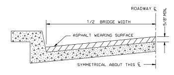
FOR BRIDGES WITH FLOOR DRAINS, CARE SHALL BE EXERCISED IN PLACING THE WEARING SURFACE AROUND FLOOR DRAINS SO AS NOT TO HINDER EFFECTIVE DRAINAGE. ALL DRAINS SHALL BE LEFT OPEN.
