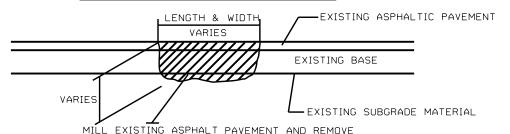
EXISTING LOOSE BASE AND/OR SUBGRADE MATERIAL AND REPLACE WITH ACIC
