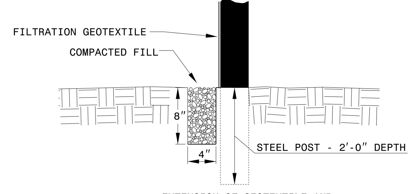
EXTENSION OF GEOTEXTILE AND WIRE INTO TRENCH
