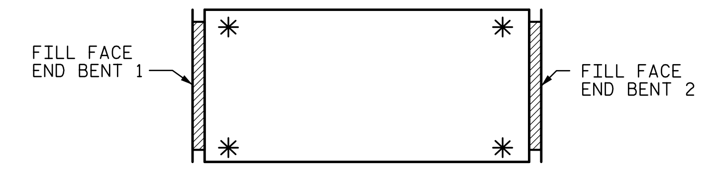
SKETCH SHOWING POINTS OF ATTACHMENTS * DENOTES GUARDRAIL ANCHOR ASSEMBLY
