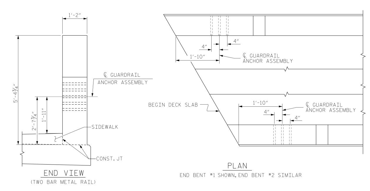
LOCATION OF GUARDRAIL ANCHOR AT END POST
